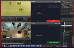
Algorithm which calculates current store occupancy and displays this in real-time along with messaging advising customers when it is safe to enter.
